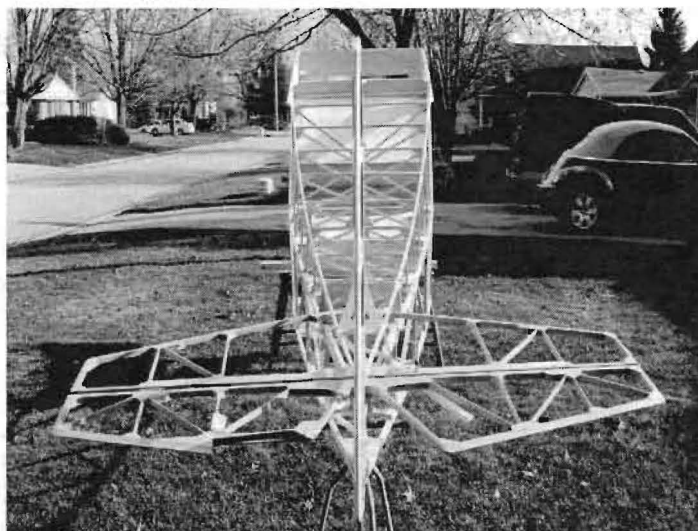
Symmetrical Fuselage. Horizontal stabilizer and elevators are just resting in place.
