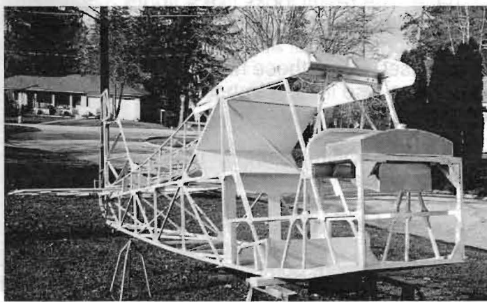
Front View of fuselage with gas tank set in place.
